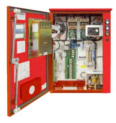
Description - Firetrol® combined automatic and manual Mark IIXG based diesel engine fire pump controllers are intended for starting and monitoring fire pump diesel engines. They are suitable for use with both mechanical and electronic type engines. The controller is available for 12 or 24 volt negative ground systems, using lead acid or Nickel-Cadmium batteries. The controller monitors, displays and records fire pump system information.
